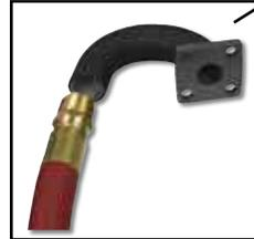
**Hose Installation:** The Series 30000 gooseneck is easily removed from the reel for hose attachment. Simply remove the four fasteners attaching gooseneck to reel, connect hose to the gooseneck and re-connect to the reel. **NOTE:** Do not discard the O-ring; insure that the O-ring is properly fitted into the grooves when replacing the gooseneck.
