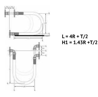
Penflex corrugated hose is engineered to provide maximum service life when properly installed. Improper installation, incorrect flexing or careless handling in an application will reduce the effective service life of the hose and cause premature failure of an assembly. The following installation and handling precautions should be observed to achieve optimum performance from your corrugated hose assemblies.
