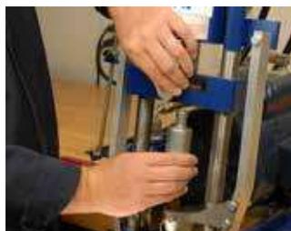
5. Insert the specified die and pusher into the swaging machine.
