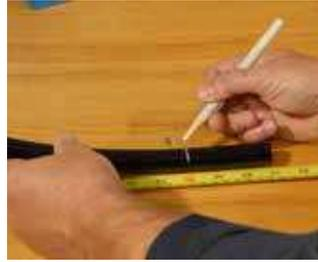
2. Use the table (to the right) to establish the length of hose that is inserted into the fitting socket. Use a rule for measurement and mark the hose with a colored pencil.
