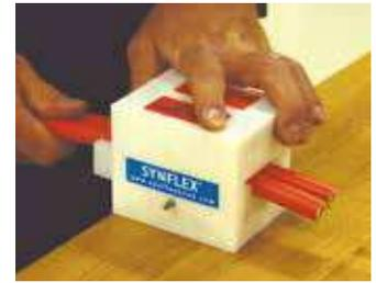
1. The De-Twiner tool 4574-01000 is designed to split twinned hose without any damage to the hose. Selecting the proper die is critical to operating this tool safely. The proper die can be selected from the provided chart. Customer service can assist in proper die selection. The hose should fit snugly in the die without extra play.
