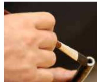
3. Lubricate inside hose diameter with SAE 20 oil.
