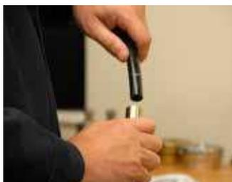
4. Insert hose into fitting to depth mark. (Use vise block 4504-00000 or 4504-01000 and rubber mallet to ease assembly.)
