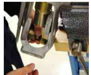
6. Place one die half into the base plate. **Lightly oil the inner surface of both die halves with SAE 90 gear oil. For stainless steel fittings use swage lubricant 4545-01001.**
