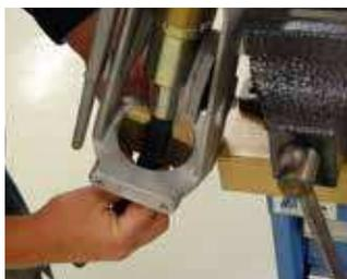
7. Insert the assembled hose and fitting through the base plate and firmly into the pusher cavity. Place the other die half in base and lock into place by swinging clamps down firmly against top of dies. Rotate ball screw until fitting reaches the die.
