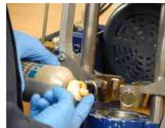
6. Lubricate die swaging surface with SAE 90 gear oil. For stainless steel fittings use swage lubricant 4545-01001.
