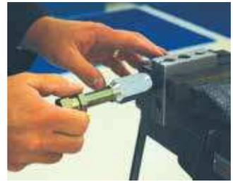
6. Remove hose and fitting assembly from vise block.
