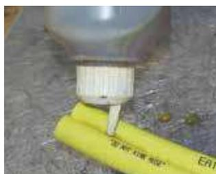
3. Lightly lubricate the hoses on both sides at the connecting web with a soap solution or lubricating oil. This step reduces friction between the knife blade and hose cover surfaces, plus keeps the knife centered during the cutting step.
