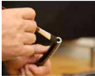
4. Lightly lubricate the outer surface of the hose to make it easier to push the fitting over the hose. For mild steel fittings and standard hose, use SAE 20 motor oil. For stainless steel fittings use swage lubricant 4545-01001\*.
