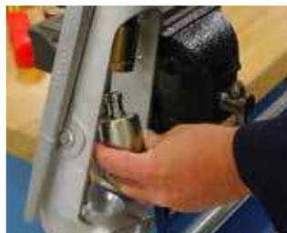
5. Insert the specified pusher with the pusher retainer in the raised position. Fingertighten retaining screw to hold pusher firmly in place. Pusher must be allowed to rotate freely.
