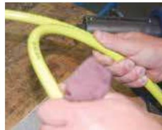
7. Examine the hose cover material where the hoses were attached to ensure they have not been cut, or the reinforcement fiber exposed. If the hose covers shows signs of damage, the hose assembly should not be placed in service. If no damage is apparent, proceed with normal hose assembly.
