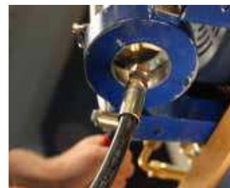
9. Push control lever to retract pusher and open die halves. Remove swaged hose assembly.
