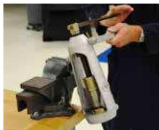
8. With handle provided or 1-1/8 socket and ratchet, rotate screw clockwise until pusher bottom contacts top of die. Maintain pressure on ball screw and release die clamps. Slowly release pressure and rotate ball screw counterclockwise until it is clear of the die. Remove swaged assembly.
