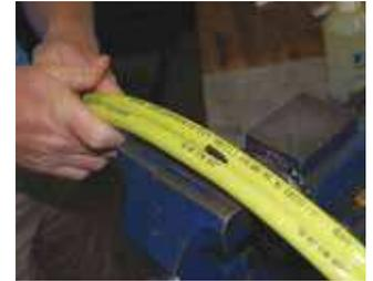
5. Hold the hoses together and aligned with the blade while first pushing then pulling them to the mark, taking care not to cut the hose covers.
