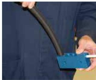
2. Mark hose for proper insertion depth into fitting. Use insertion depth chart or use insertion depth marker 45J0-04603.
