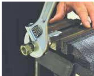
8. Screw the fitting insert clockwise into the socket with a wrench until the bottom of the inserted hex contacts the socket shoulder. Do not over-tighten.
