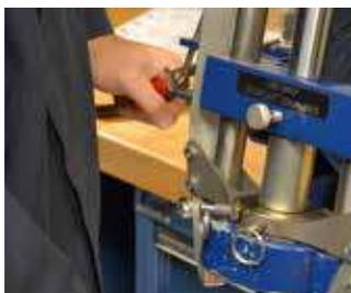
8. Pull control lever and guide fitting into the die until the pusher bottom is against the top of the die surface.
