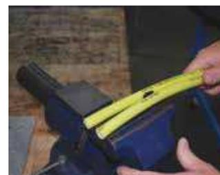
4. Push the hose into the "V" notch on the knife blade using a rocking motion to start the hoses into the blade.
