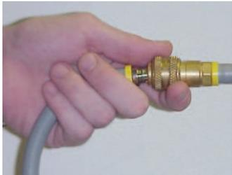
After pulling the sleeve, the nipple will move out of the coupler slightly. Continue to hold the hose and coupler sleeve until all air is fully exhausted.
