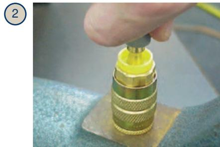
2 Place the end of the fitting against a flat object and grip the hose one inch from end. Push with a steady force until end of hose is covered by yellow plastic cap.
