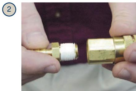
Check threads to make sure there is no obvious damage on either half and that tape is properly installed. Align male and female threaded connections and carefully begin threading the two halves together.
