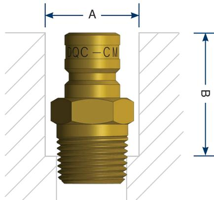
Counterbored mold ports will protect the male threaded nipple, allowing the nipple to be mounted below the surface, simplifying storing and handling of molds. Dixon male threaded plugs are constructed of corrosion resistant brass to maximize longevity in moist environments.
