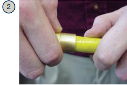
2 Install ferrule by slipping it onto the end of the hose and twisting it counter-clockwise.
