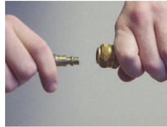
After the line is fully exhausted, you are able to safely separate the nipple from the coupler.
