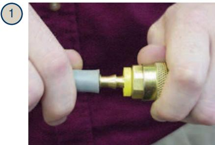
1 Trim hose end squarely and lubricate the Push-Loc barb and hose. Insert Push-Loc barb into hose until first barb is in the hose.
