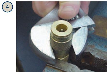
4 Turn the reusable fitting into the ferrule until coupling is seated against ferrule.
