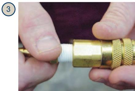
Finger tighten the connection and create a reference mark on the hex of the hose end/adaptor and the coupling. This mark will help identify the number of revolutions during the next step in the procedure.
