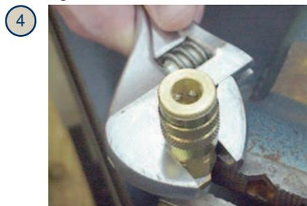
With even and smooth force applied, wrench tighten according to the 'Turns From Finger Tight' (T.F.F.T.) values listed below. **DO NOT OVERTIGHTEN!**
