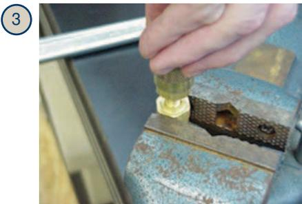
3 Apply lubricant sparingly to the reusable barb before inserting it into the ferrule.
