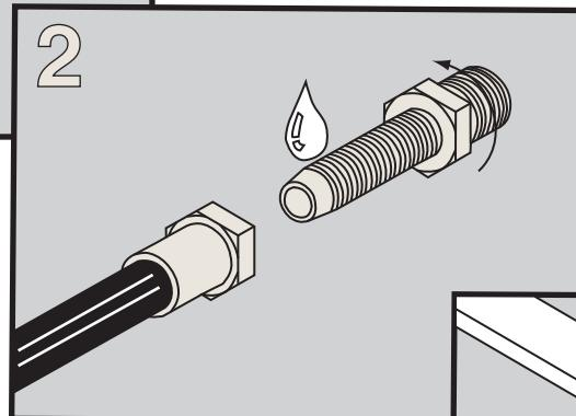
Apply a drop or two of lubricant to fitting before inserting ferrule.
