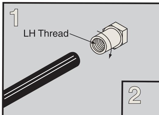
Simply slip and twist ferrule on end of hose which has been trimmed flush. No skiving necessary.
