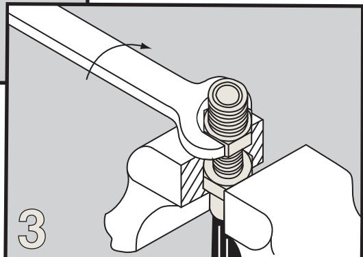
Turn reusable fitting into ferrule. Hose is expanded inside ferrule for perfect fit.
