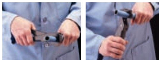
The rotating/rocking technique produces fast easy cuts.
